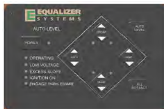
Hydraulic Control Panel
