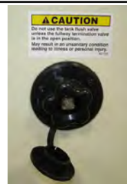
Tank Flush Inlet
